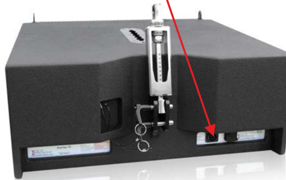
Ikkarray-12 bi-amping LF 12" an CH1, 2400W, Speakon 2+/- HF 1,4" an CH2, 800W, Speakon 1+/-
